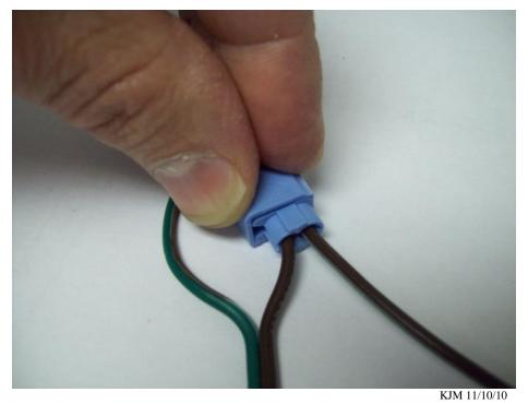
Close the hinge cover on the connecter, this finishes the process. This illustration is used in the next step for wiring the side marker lights.
